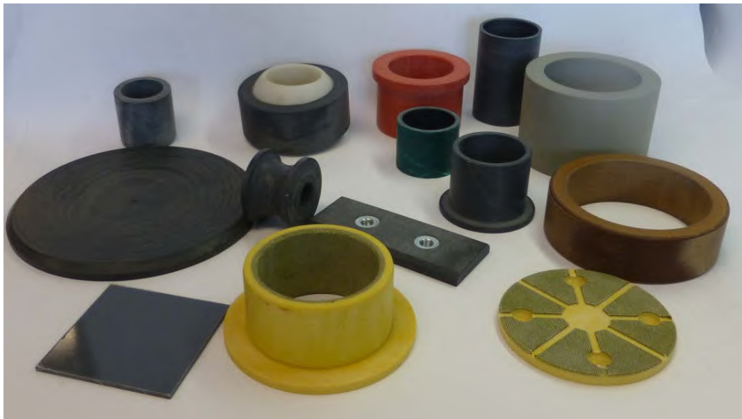
Figure 12-2. Textile-Reinforced Resin Self-Lubricated Materials.
