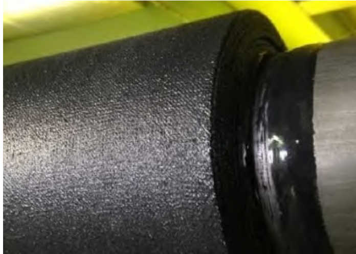
Figure 12-5. Cured Material on Mandrel.
