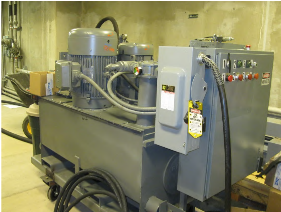
Figure 10-2. Cleaning and Flushing Unit for Hydraulic Systems.
