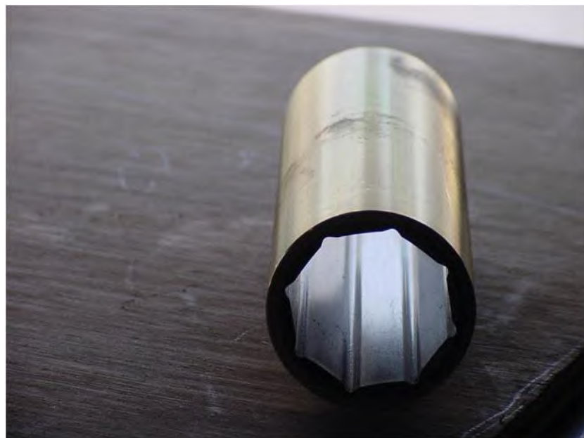
Figure 12-34. Water Lubricated Bearing.
