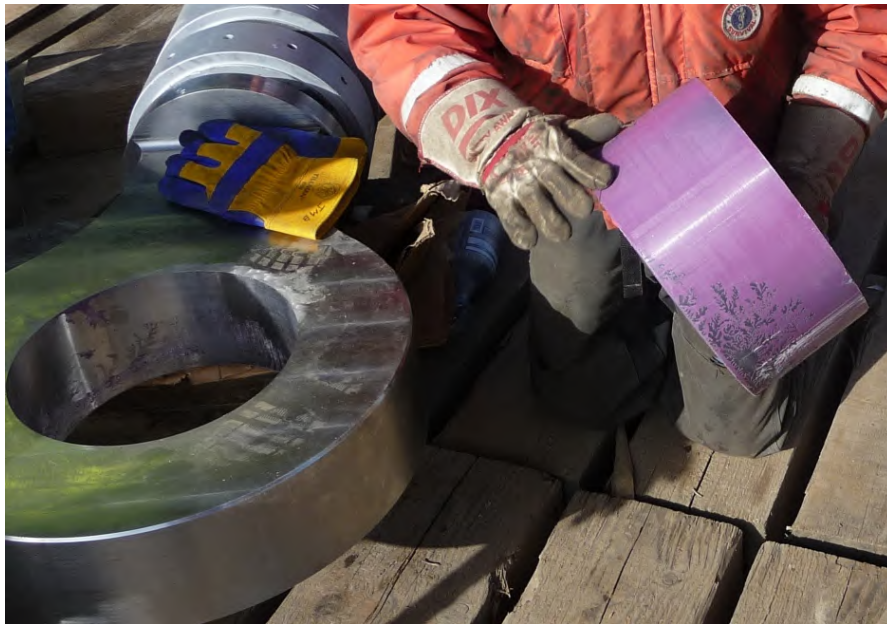
Figure 12-17. Disbonding Failure from Improper Housing Surface Preparation.
