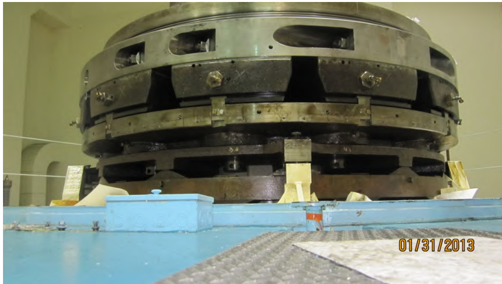
Figure 9-2. Tilting Pad Thrust Bearing Assembly
