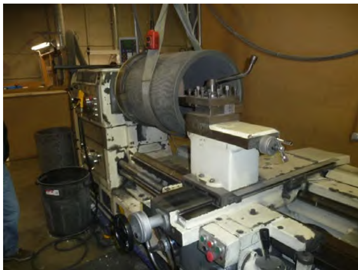
Figure 12-6. Machining of Fabric-Reinforced Resin Materials.
