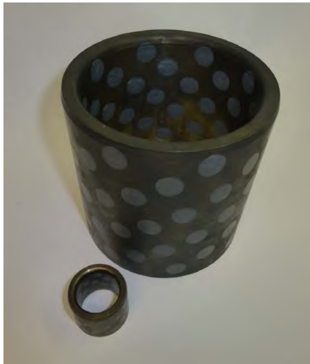
Figure 12-14. Plugged Metal Self-Lubricated Materials.
